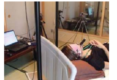
Measuring how easy it is for women to hold the digital thermometer in the mouth in a simulation home environment
