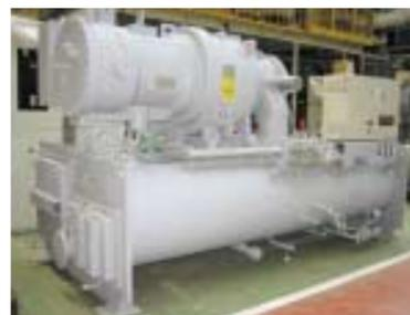
The high-efficiency turbo refrigeration unit (Kofu Factory)
